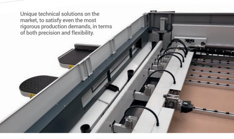
The **presser** boasts a single-element structure which guarantees consistent, controlled pressure on the book of panels to be cut. The opening is automatically optimised according to the thickness of the book of panels, in order to achieve the best cut quality and to reduce cycle times.
