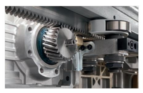
The perfectly linear movement of the tool holder carriage is achieved through a helical rack and pinion system and is driven by a brush-less servomotor.
