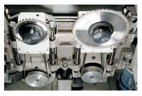
The superior cutting quality is achieved through independent rise and fall movements of the main blade and the scoring blade.
